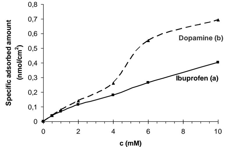
The plasmonic curves of adsorption of (a) ibuprofen and (b) dopamine on gold surface at different concentrations (0.5, 1, 2, 4, 6, 10 mmol/dm<sup>3</sup> aqueous solutions)
