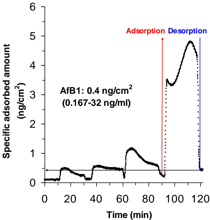
**Fig. 7.** Results of SPR measurements: AfB1 solution (0.167-32ng/ml) to gold surface.
