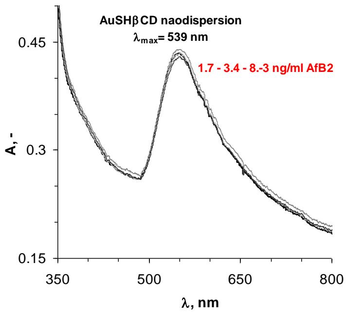
The changes of plasmon bands of AuSH $\beta$ CD gold nanodispersions (164 mg/ml; 0.5 mM Au) added AfB1 (in concentration range 3-33 ng/ml AfB1 and 1.7-8.3 ng/ml AfB2) to the solution are also registered by UV-Vis spectroscopy in dilute acetonitrile solution.
