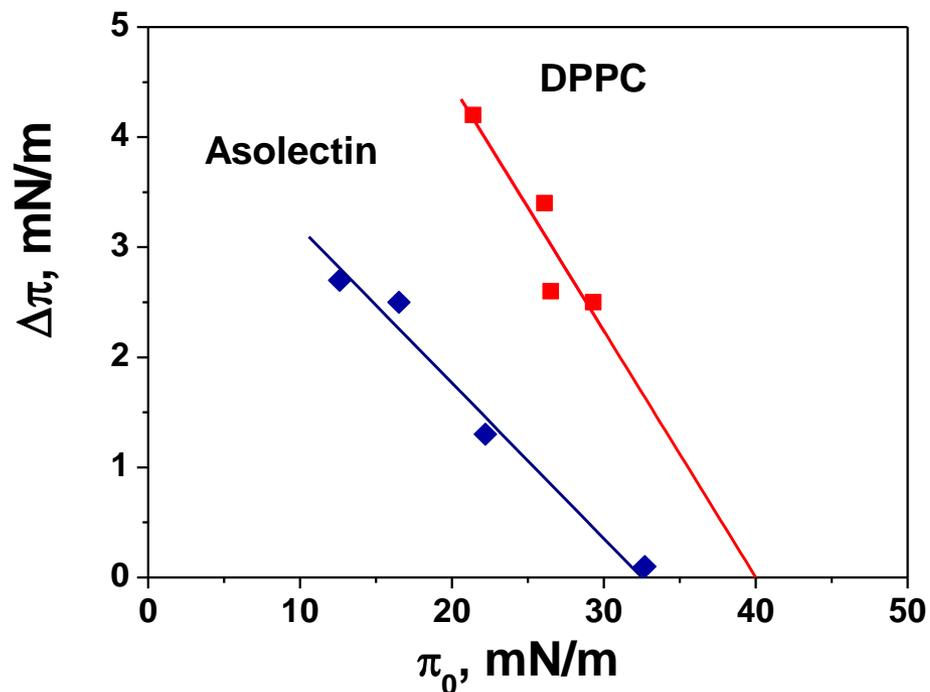
Surface pressure increase ( $\Delta\pi$ ) as a function of the initial surface pressure ( $\pi_0$ ) due to the nanoparticle incorporation
