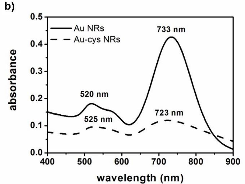
TEM image of the Au nanorods, UV-Vis absorbance spectra of the aqueous dispersions of the Au NRs.
