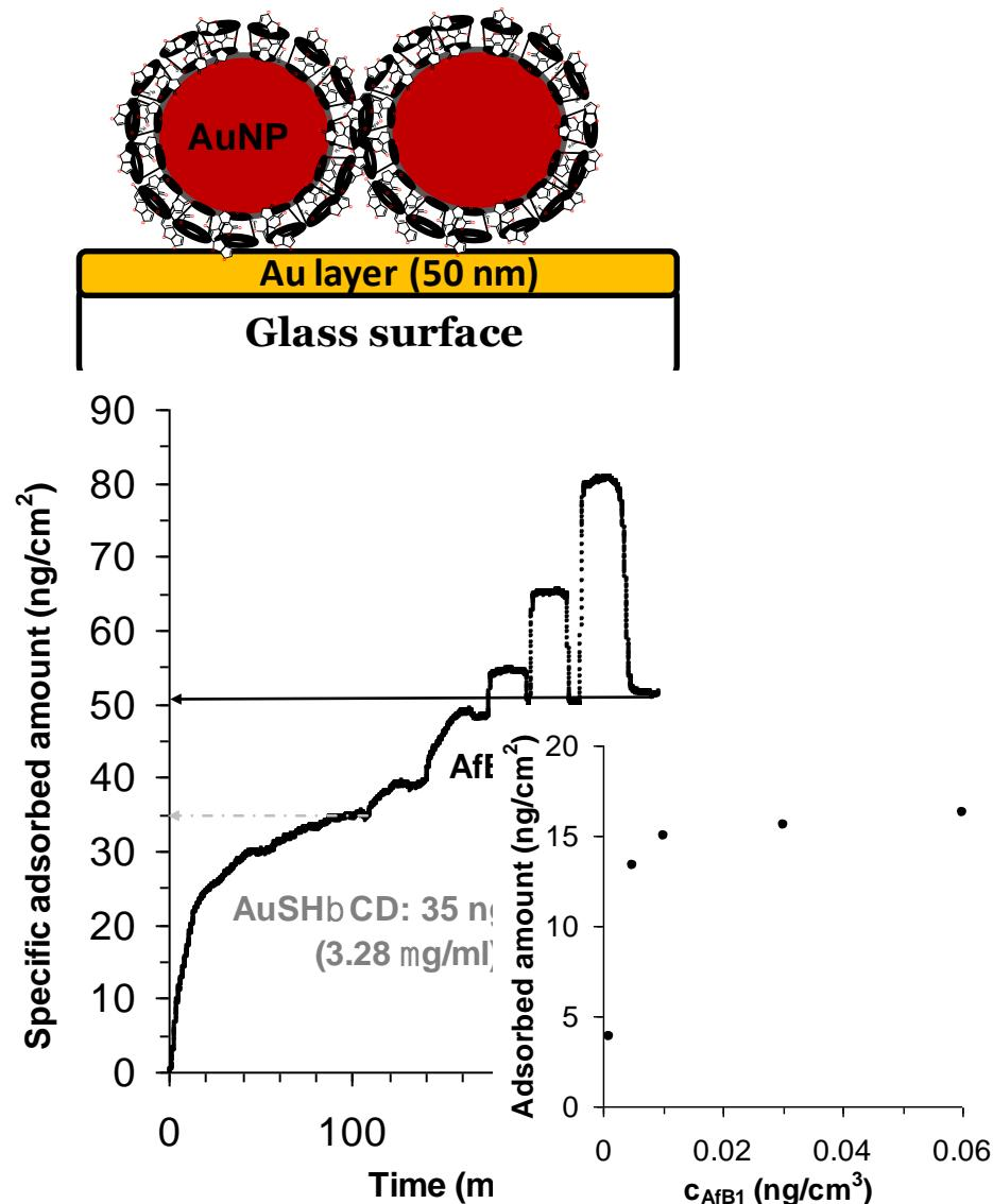
**Fig. 11.** Results of SPR measurements: in first step Au nanodispersion and after added AfB1 (in concentration range 0-32 ng/ml AfB1) in dilute acetonitrile solution.
