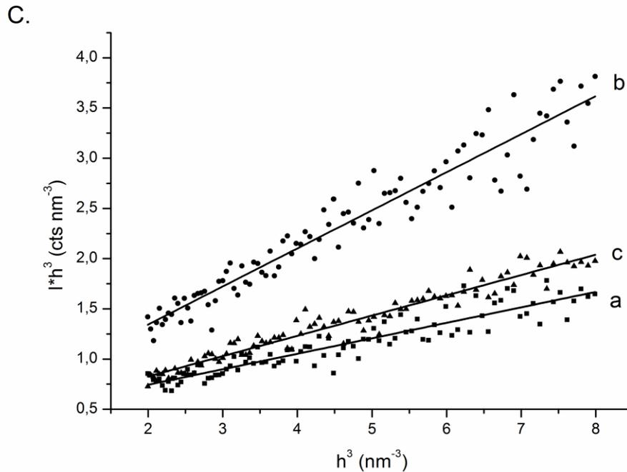
(A) The SAXS curve of the AuNP(Lys) nanoparticles in Kratky representation (B) calculated pair distance distribution function of the AuNP(Lys) samples  $m_{\text{Lys}}/m_{\text{Au}} = 5$  (C) the SAXS curves of Porod representation  $m_{\text{Au}}/m_{\text{Lys}} = 1:5$  (a), 1:15 (b), 1:20 (c)
