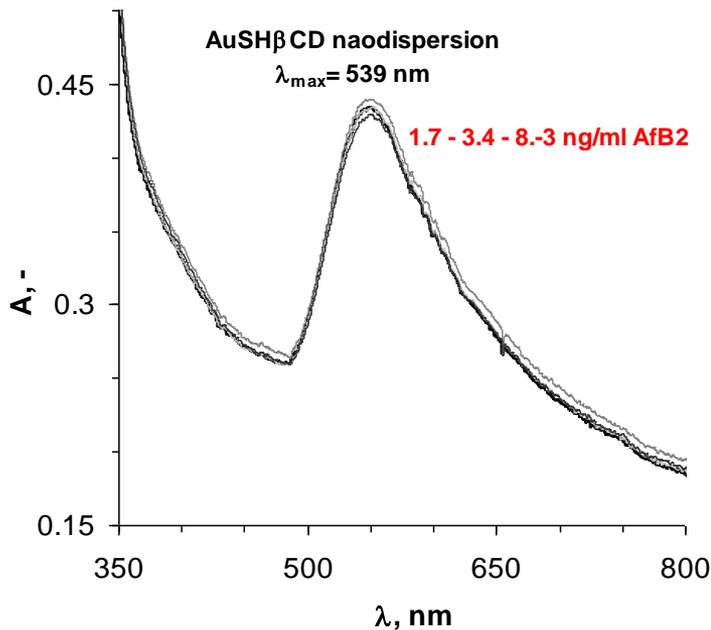
The changes of plasmon bands of AuSH $\beta$ CD gold nanodispersions (164 mg/ml; 0.5 mM Au) added AfB1 (in concentration range 3-33 ng/ml AfB1 and 1.7-8.3 ng/ml AfB2) to the solution are also registered by UV-Vis spectroscopy in dilute acetonitril solution.
