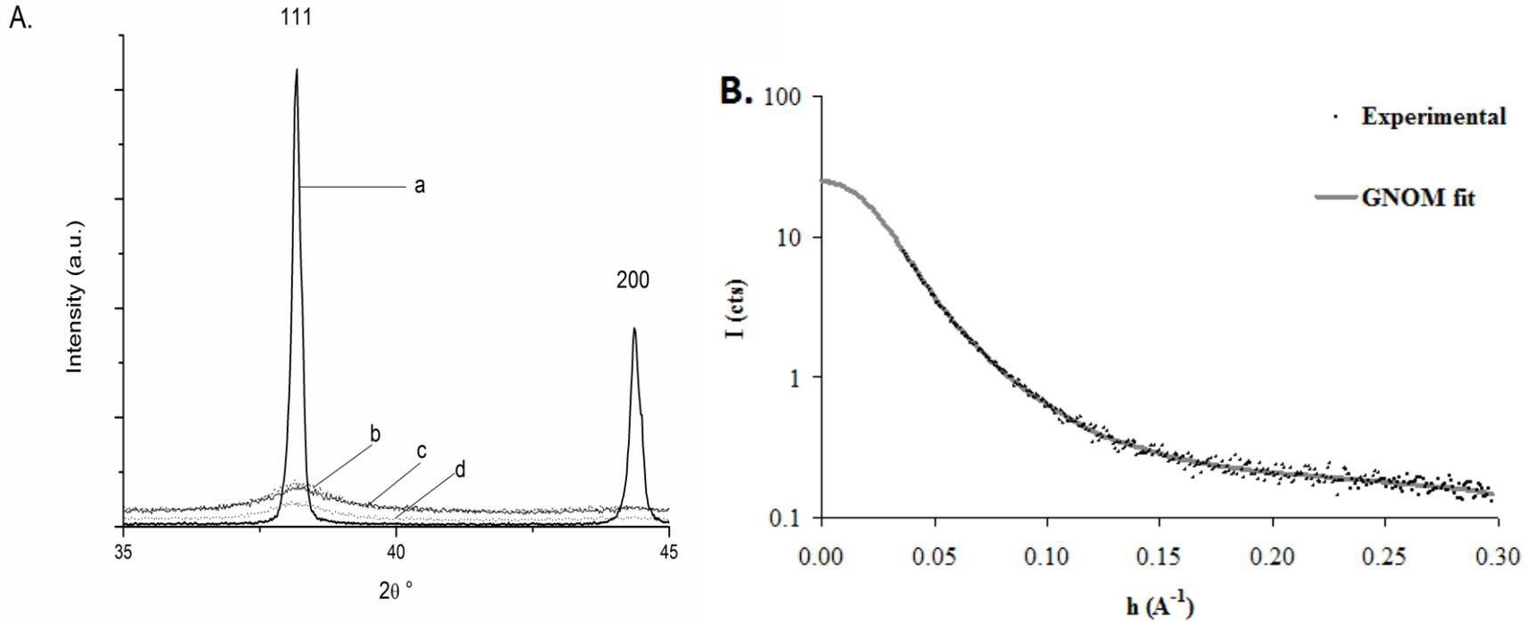
(A) XRD pattern of (a) bulk gold, (b) AuNP(cit), (c) AuNP(Lys) and (d) AuNP(Cys) samples (B) The SAXS curve of (a) AuNP(Lys) sample ( $c_{\text{Lys}}=1$  mg/ml) and the calculated SAXS curve (GNOM fit)
