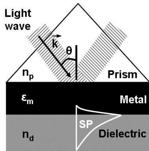
The prism coupling (Kretschmann-configuration) in SPR technique
