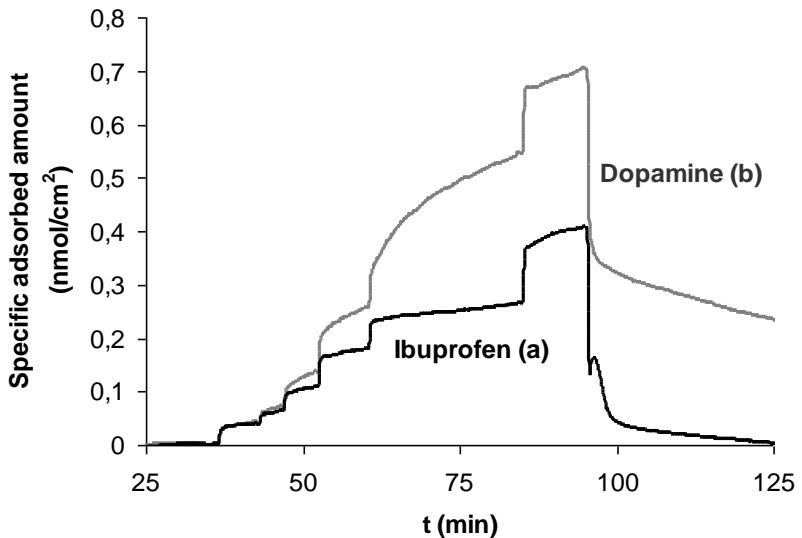
The plasmonic curves of adsorption of (a) ibuprofen and (b) dopamine on gold surface at different concentrations (0.5, 1, 2, 4, 6, 10 mmol/dm<sup>3</sup> aqueous solutions)
