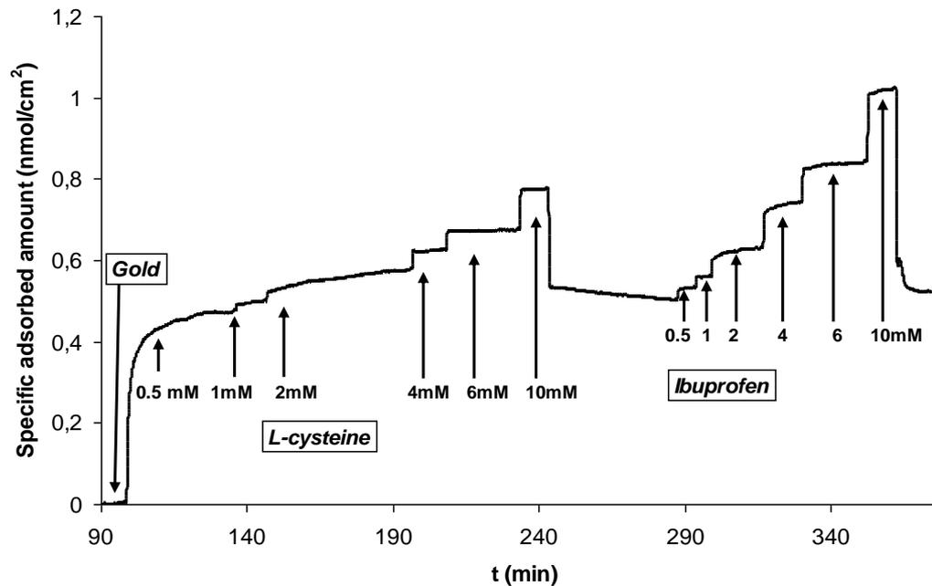
The plasmonic curves of adsorption of ibuprofen on L-cysteine functionalized gold surface from aqueous solutions ( at 0.5, 1, 2, 4, 6, 10 mmol/dm<sup>3</sup> concentrations )
