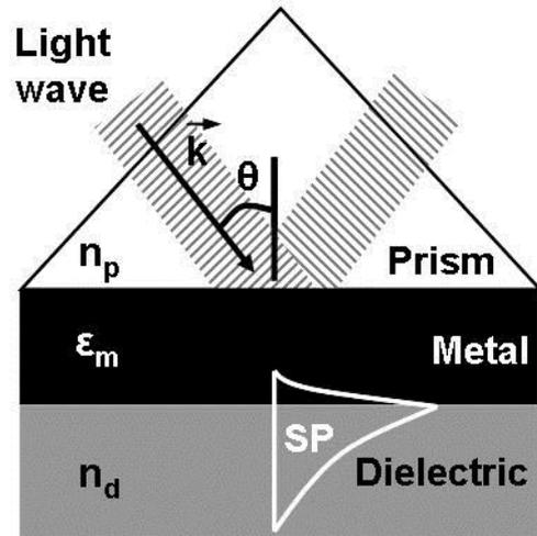
The prism coupling (Kretschmann-configuration) in SPR technique
