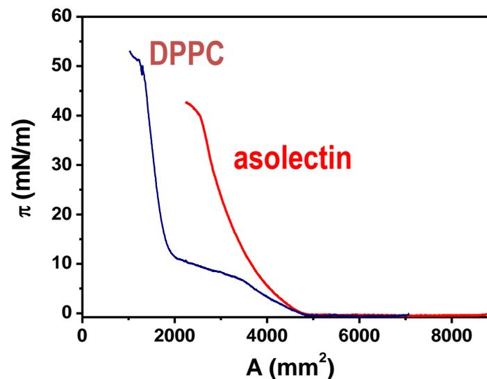
Surface pressure – area isotherms of the model membrane materials: DPPC and asolectin
