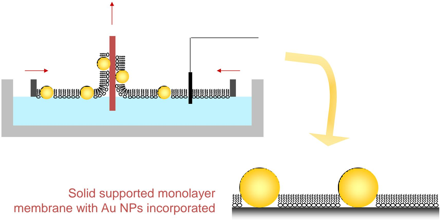
Solid supported monolayer membrane with Au NPs incorporated
