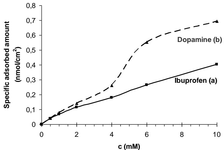
The adsorption isotherm of (a) ibuprofen and (b) dopamine from aqueous solution on gold surface
