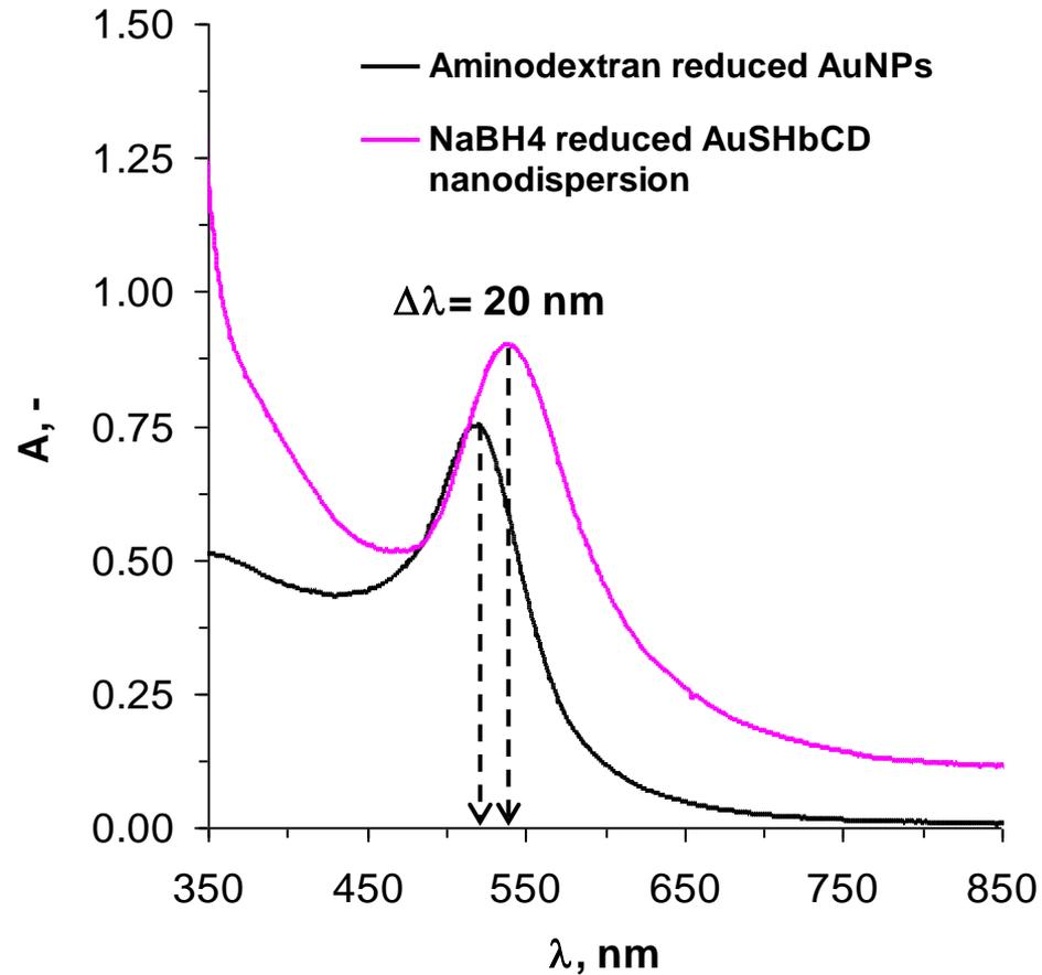
The changes of plasmon bands of aminodextran reduced gold nanodispersion and AuSH $\beta$ CD gold nanodispersions (164 mg/ml; 0.5 mM Au) registered by UV-Vis spectroscopy.
